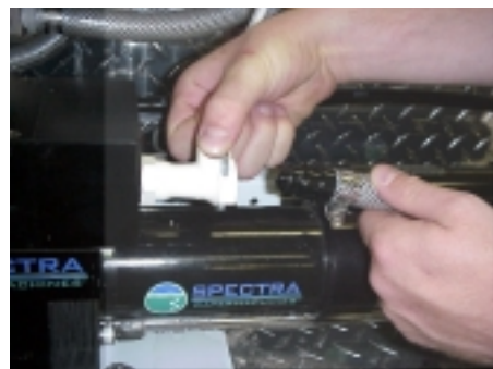
Connecting brine discharge hose
