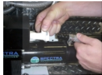
Connecting the brine discharge service hose
