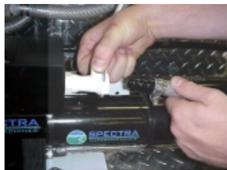
Connecting brine discharge hose
